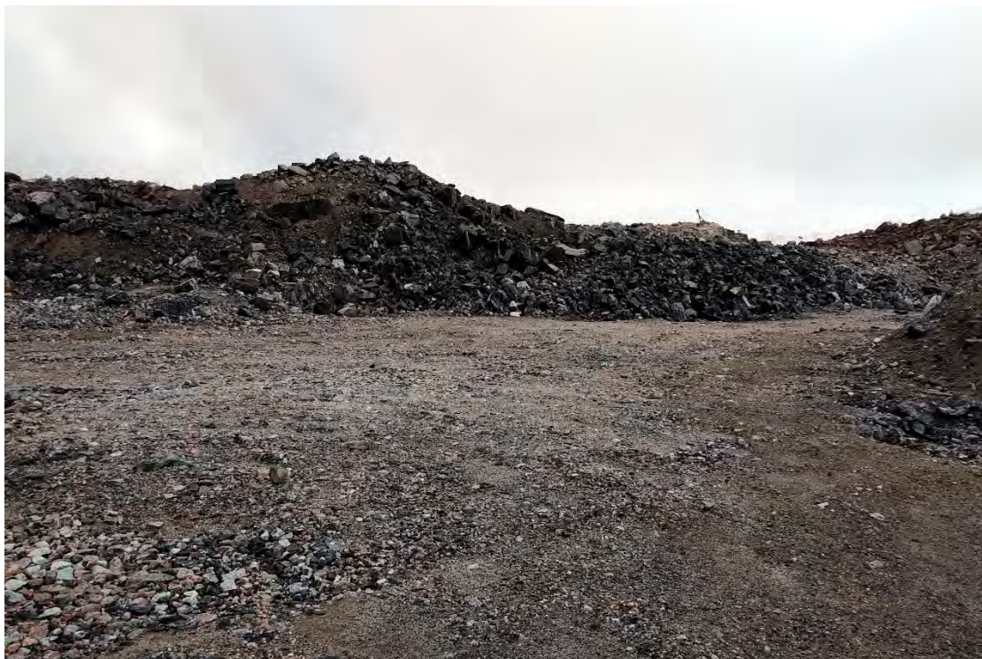
Photo 1: Site 1- Kudlik Quarry - Blasted rock stockpiled Ready for Crushing
