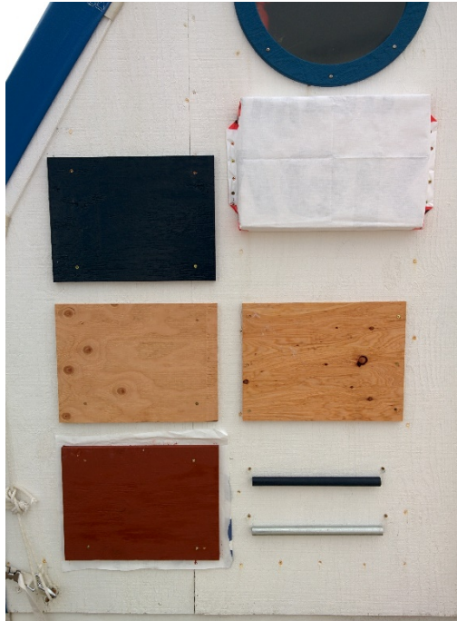
Figure 6. Material samples installed for weathering tests on end wall of technology tent. Left, from top: Plywood coated with (a) linseed oil paint, (b) bare, (c) pine tar. Right, from top: (d) MycoFoam insulation panel wrapped in Tyvek sheathing, (e) Plywood coated with linseed oil, Galvanized steel tubing coated with (f) linseed oil paint, (g) bare.
