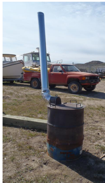
Figure 4 – Modified Burn Barrel
