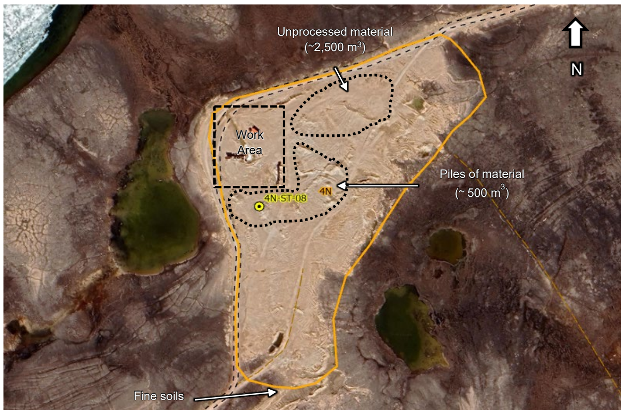
Figure 3 Remaining Volume Estimate – Existing Quarry Site 4N
