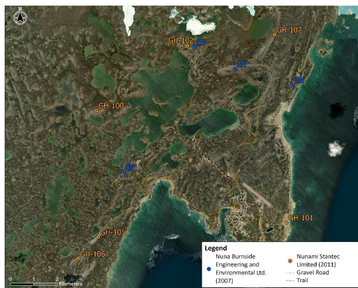
Figure 2 Potential Borrow Source Locations Identified in the Previous Aggregate Studies
