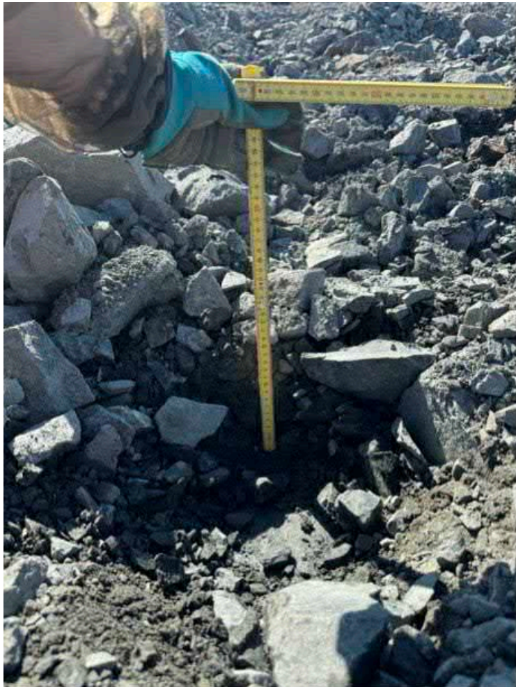
Figure 8: Example four of waste rock remaining on north ore pad area (~15 cm depth).
