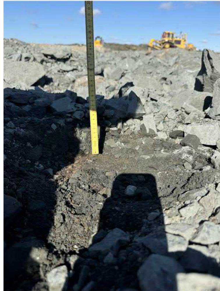
Figure 9: Example five of waste rock remaining on north ore pad area (~5 cm depth).
