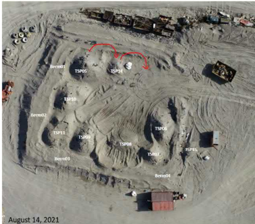
Figure 1: Aerating of stockpiles in the soil holding area August 2023.
