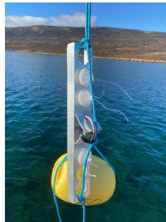
Installing a temperature logger in a river near Qik (left) and eDNA pods attached to a buoy (right)
