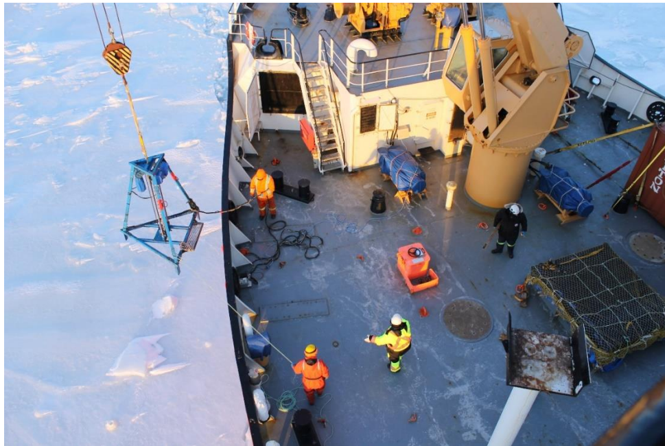
Figure 1: RapidCore being deployed in level ice from the CCGS Henry Larsen.
