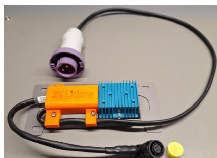
DC/DC Power Supply
