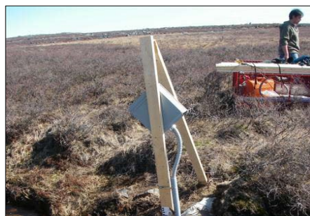
A hydrologic monitoring station installed at station R1 (left) and obtaining manual flow measurements at station W2 (right).
