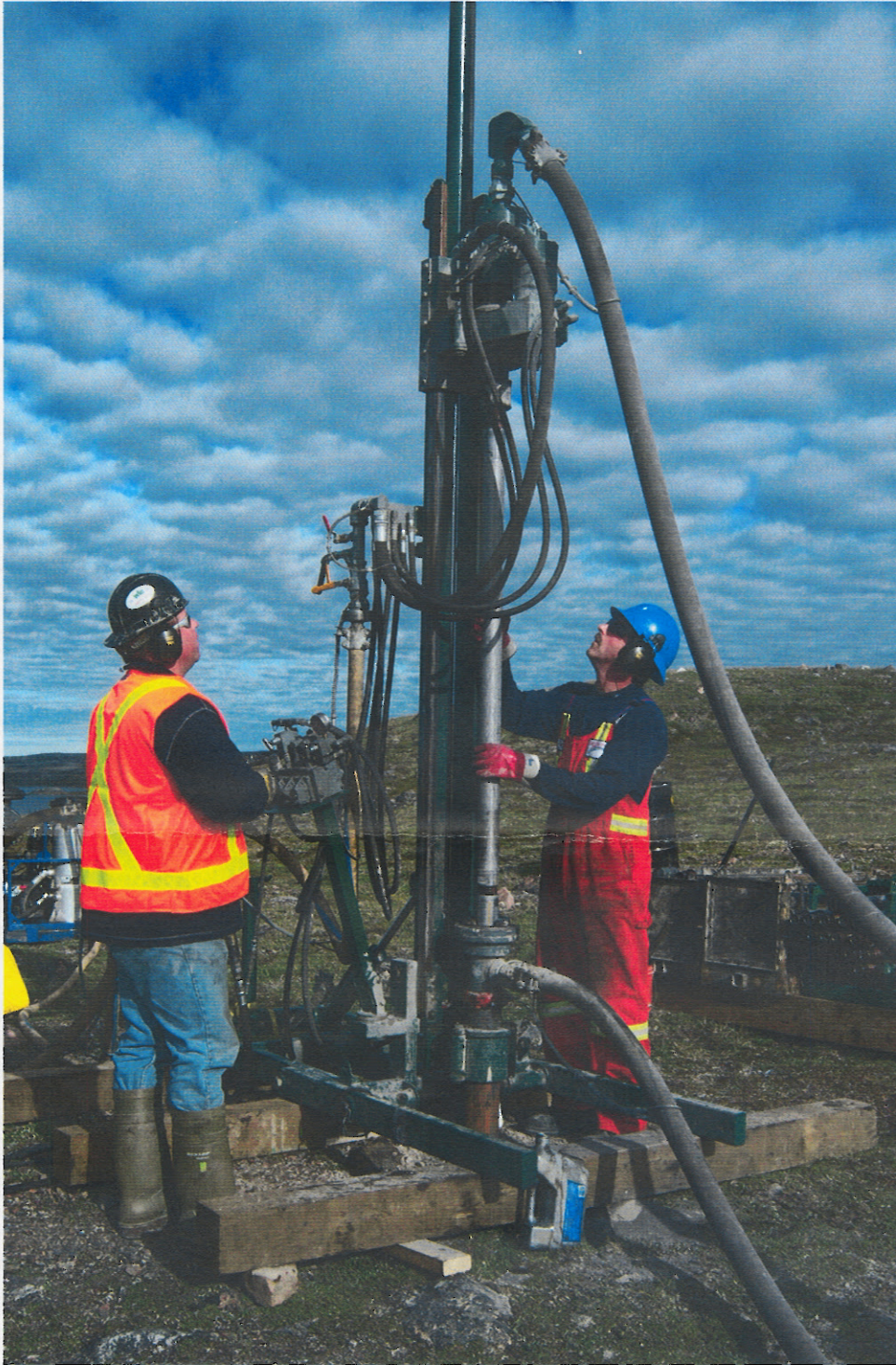
Reverse circulation drill rig used at Amer Lake
