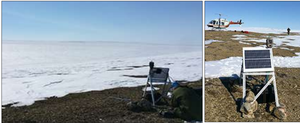
Figure 1. Outdoor digital camera and solar panel in place at Polar Bear Pass
