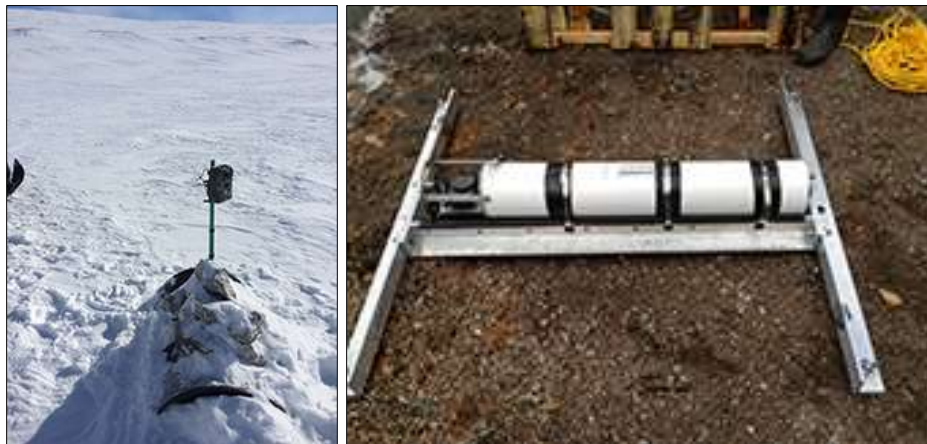
Figure 2. Outdoor camera in place at Small Lake and example of the Ice sensor currently on the bottom of the lake, with a rope floating for retrieval.
