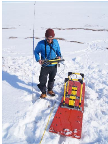
Fig. 2. Ground penetrating radar.
