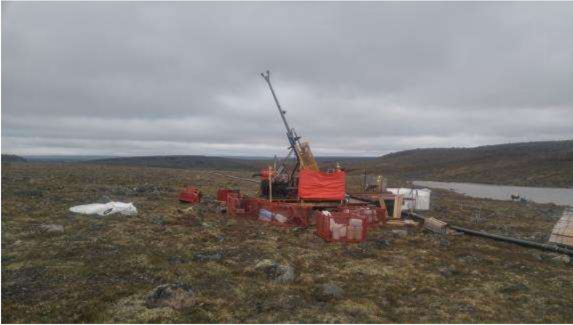
Figure 4: Diamond Drill Set Up on Pad
