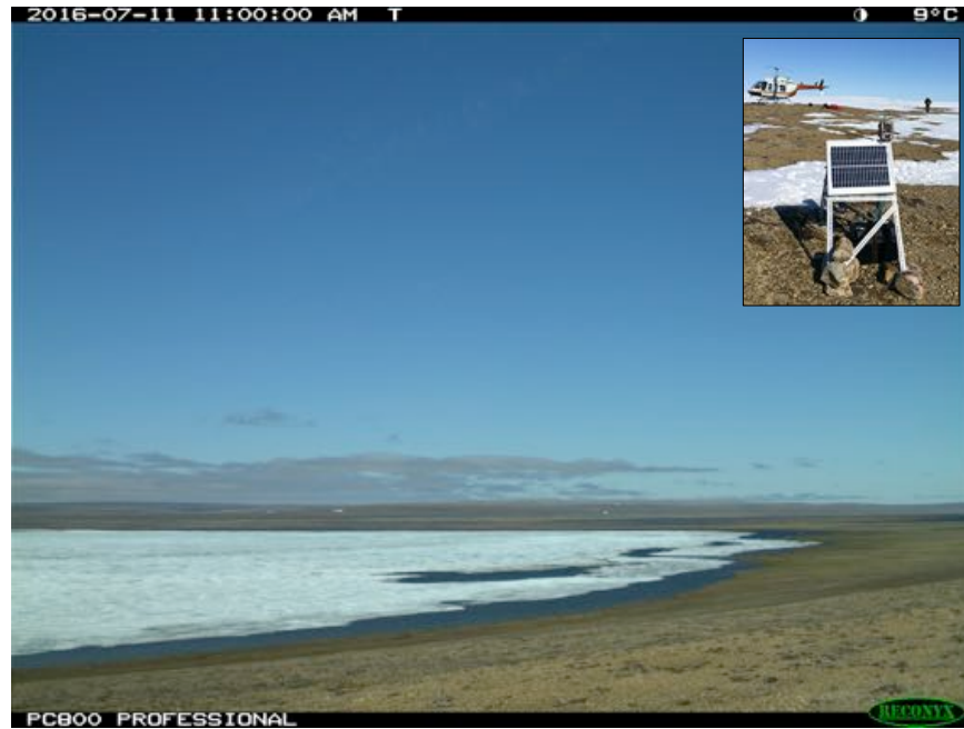
Figure 1. Outdoor digital camera and solar panel in place at Polar Bear Pass, and example picture collected showing the view of the lake ice on Hunting Camp Lake.
