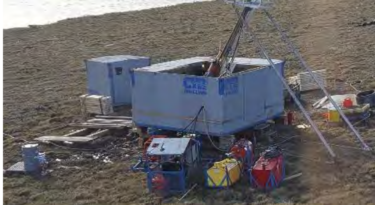
Figure 8: Drill site fuel storage - diesel in double-walled storage containers and single Jet A barrel in small berm.
