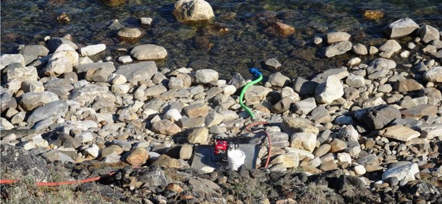
Photo 2: Water pump with intake screen in blue.
