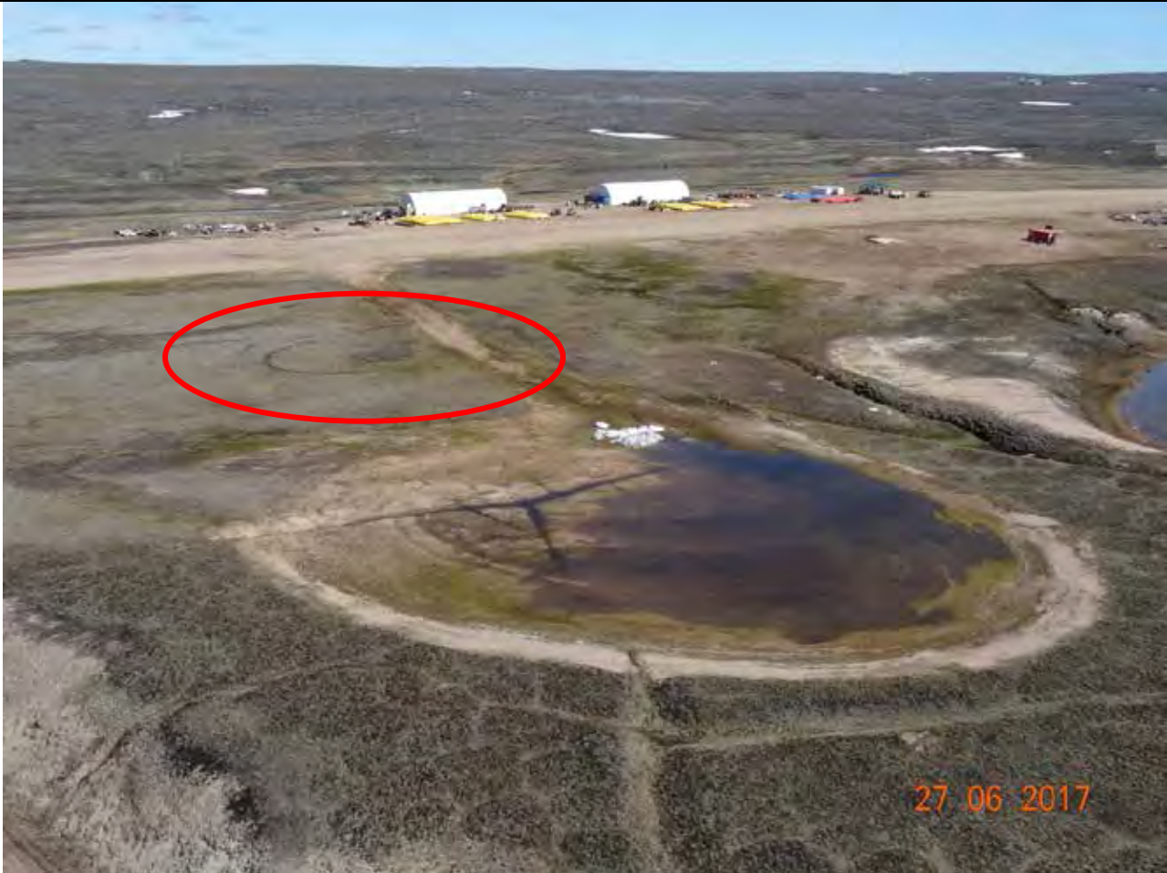
Description: Borrow Area 1 identified in expired quarry permits has not been reclaimed and is accumulating water. Historic drainage channels are evident. Sampling was done to determine whether the cuttings placed in the quarry are affecting the water chemistry. Red circle above the quarry denotes the recent ruts caused by turning the plane. This tundra is easily rutted, and further impacts are to be mitigated.
