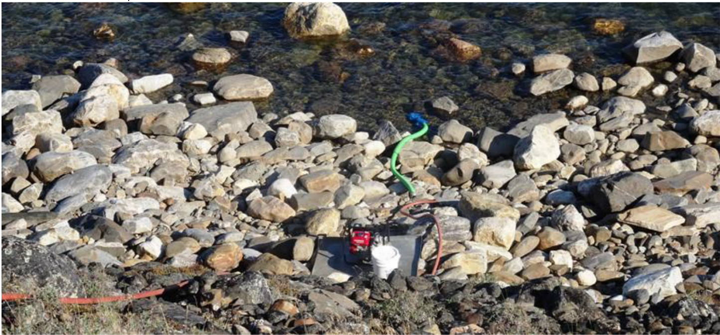
Photo 2: Water pump with intake screen in blue.
