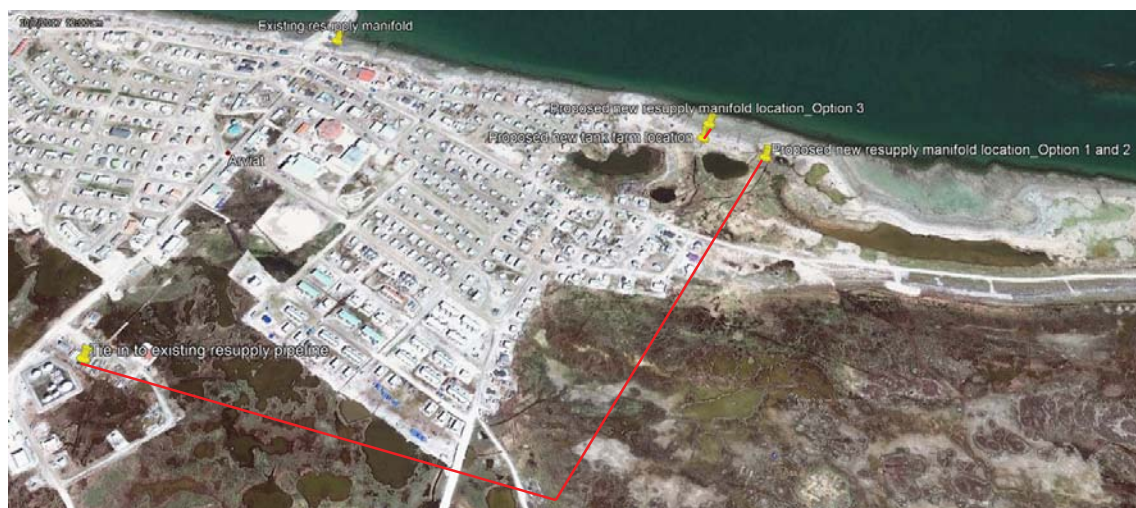
Figure 24: Proposed double-wall, underground resupply pipeline routing for Option 1 and Option 2. Leaving resupply manifold in its current location is not considered.
