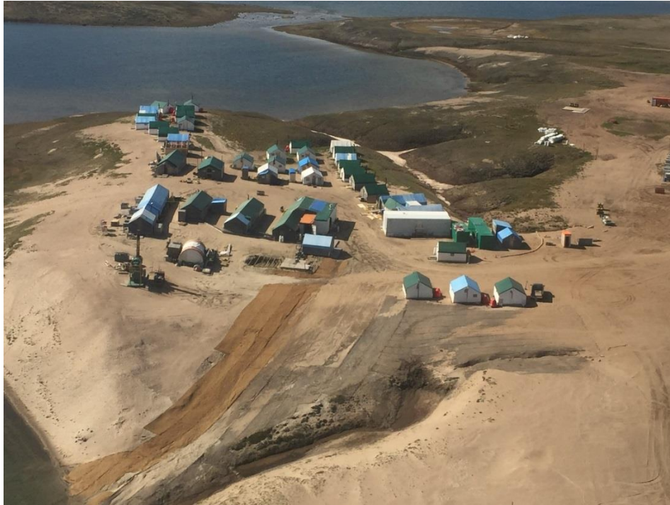
Figure 13: Additional, light coloured coconut matting installed to mitigate sand being eroded by freshet 2018 (early July 2018).
