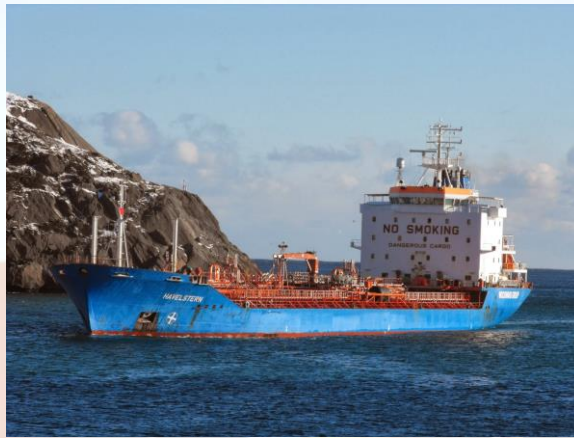
Figure 10.6: One of the ships used to haul fuel to PPD Oil Handling Facilities. The maximum oil transfer rate from vessel to fuel storage tanks in Arviat tank farm is 75 m 3 /hour. This will rate the Arviat tank farm a “ Level One Facility ”.
