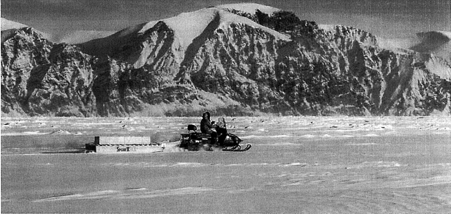
Moses Amagoalik, a SmartICE operator in Pond Inlet, measures sea-ice thickness in Eclipse Sound using the SmartQAMUTIK (March 2018). SmartICE puts into the hands of communities the tools they need to travel safely on changing sea ice. Michael Schmidt photo
