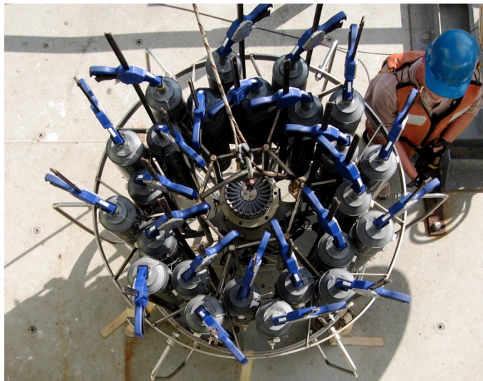
Fig. 1. Top view of rosette showing arrangements of bar clamps.
