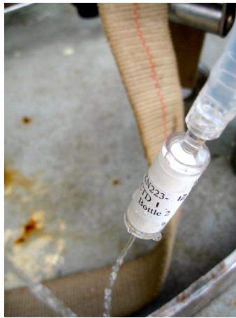
Fig. 3. Sterivex 0.2 \mu\text{m} retention filters used in-line from Niskin bottle.
