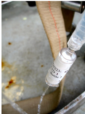
Figure A-3. Sterivex 0.2 \mu\text{m} retention filters used in-line from Niskin bottle.
