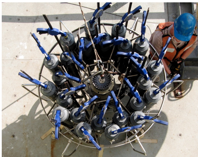
Figure A-1. Top view of rosette showing arrangements of bar clamps.
