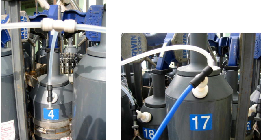
Figure A-2. T-fittings used to plumb pressure manifold to Niskin bottles.
