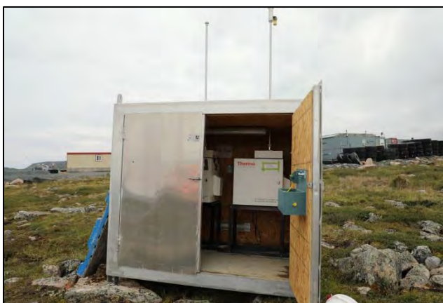
Photo 45: Air and partisol monitoring station near the emulsion station
