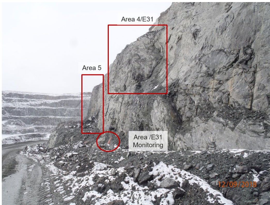
Photograph 6-21: Area 4/Zone E31 crack meter monitoring
