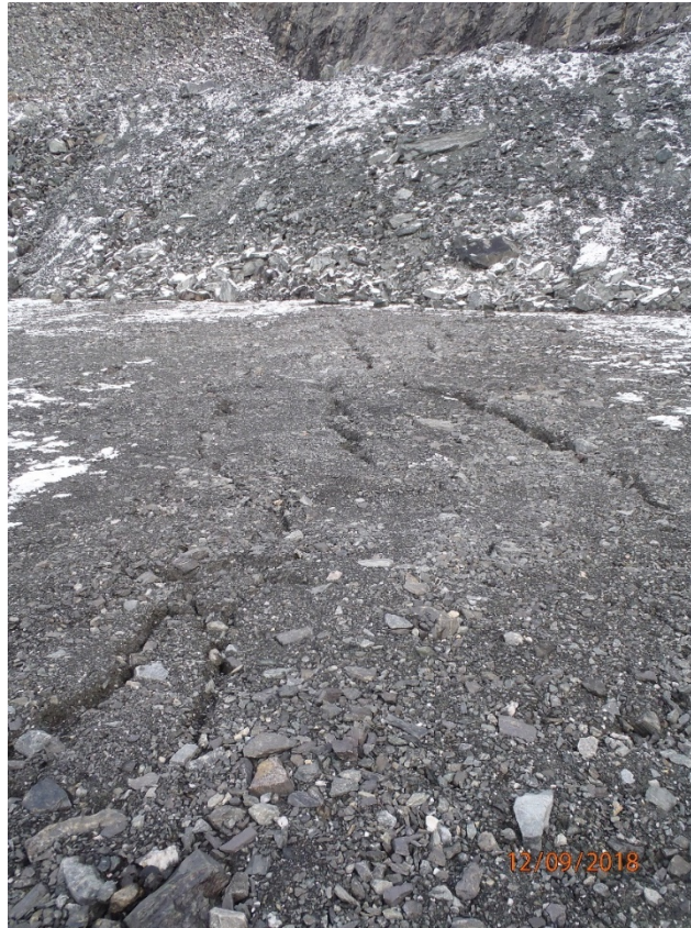
Photograph 5-4: D Dump radial tension cracks
