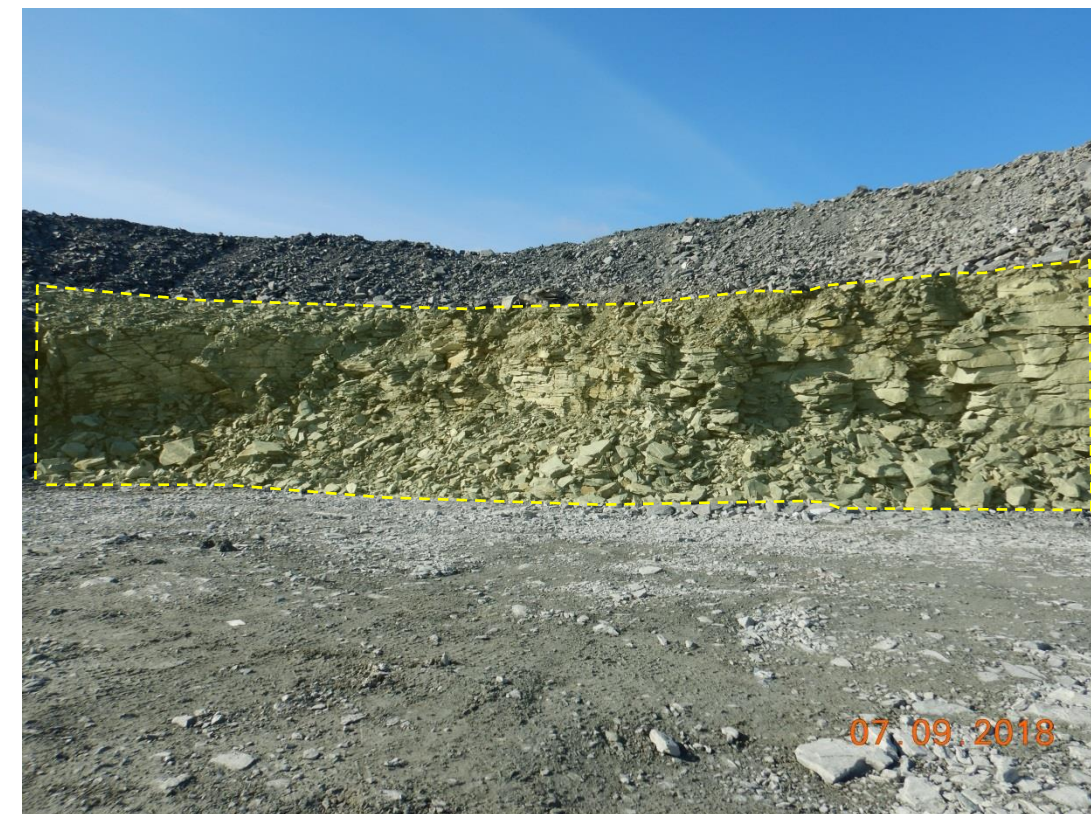
Zone BB04: E4, West Wall: Lightly scale the wall, and pick up debris.
