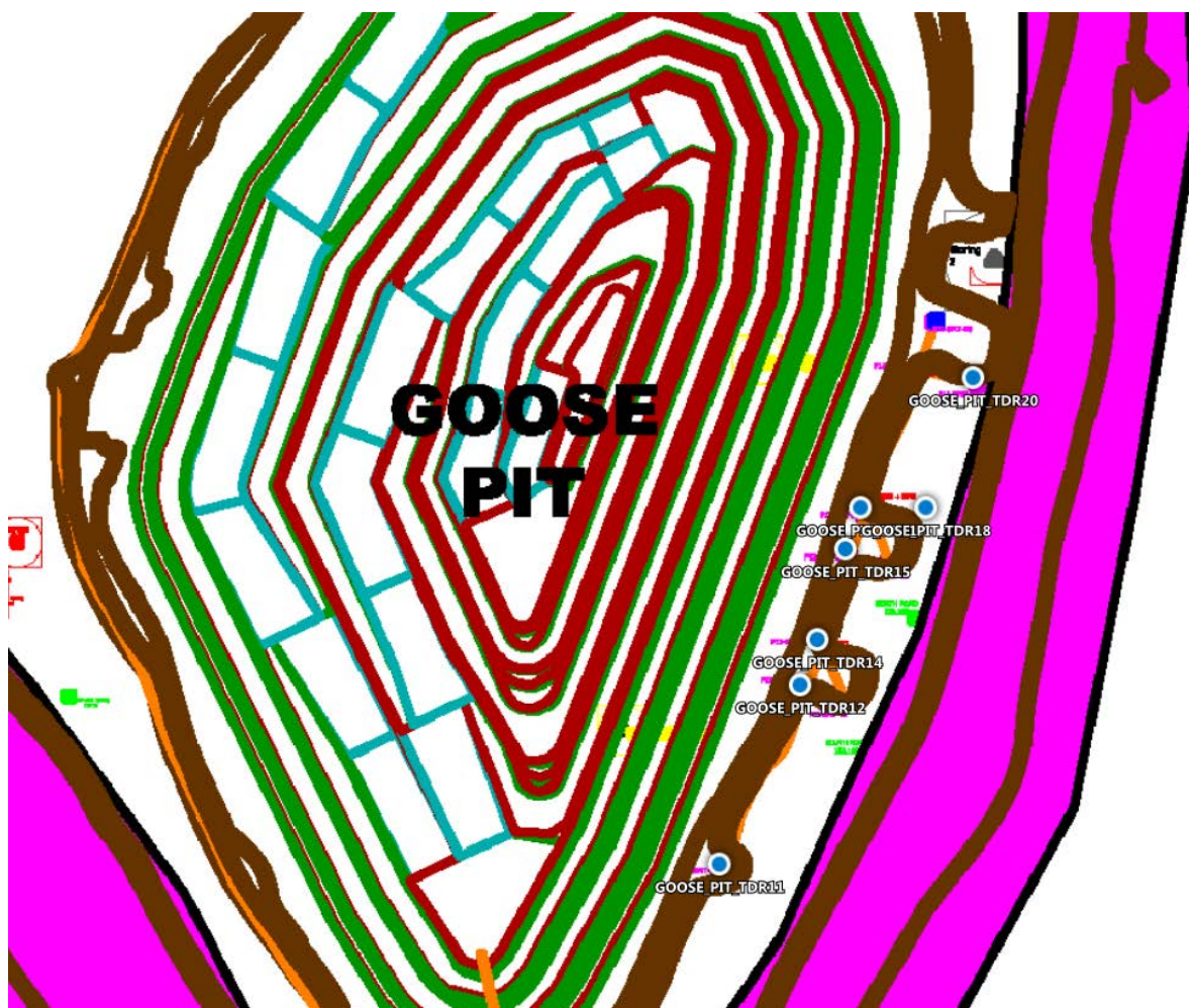
Figure 7: Location of downhole instruments at Goose pit
