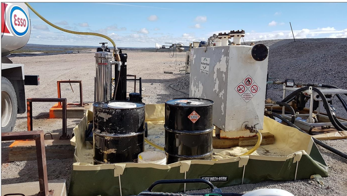
Photo 22: ROJV Fuel Filtration System
