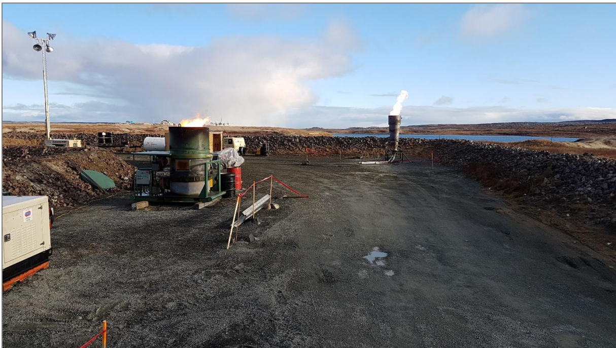
Photo 51: Second Incinerator Set-up
