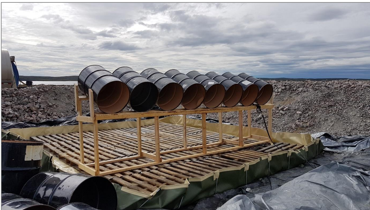
Photo 44: Drum Cleaning Set-up
