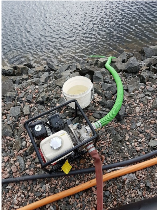
Transfer water into water truck with a small water pump (suction has a screen on it)
