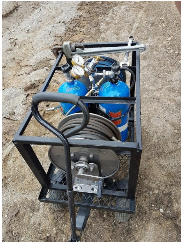
Air tanks for SABA system
