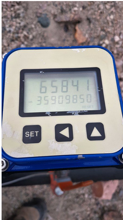
957,662gal pumped out of West dam to pit
