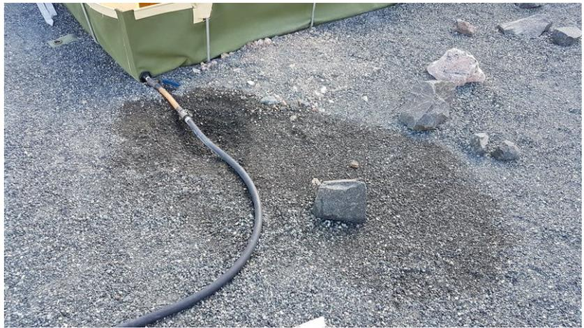
fuel berm drainage small leak
