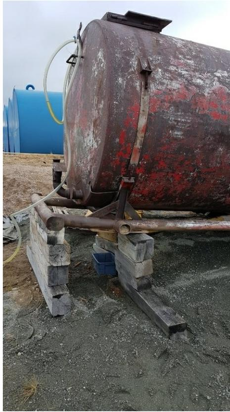
leak on the red tank while transferring into tank from the drums
