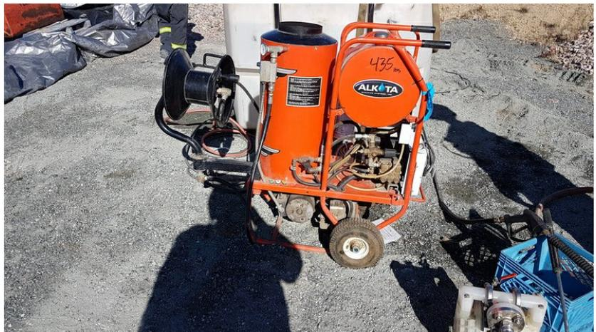
pressure washer steamer needs head pressure to pump water so it also has pressure to wash the drums
