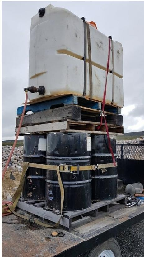
holding tank for steam cleaning
