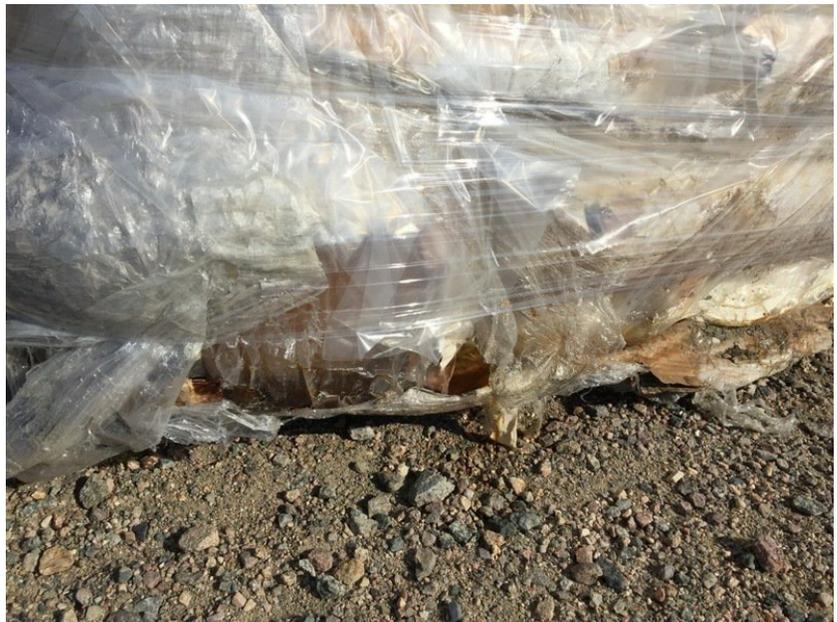
Leaking polymer at base of some pallets in poor condition. ROJV confirmed these will be placed in mega bags.
