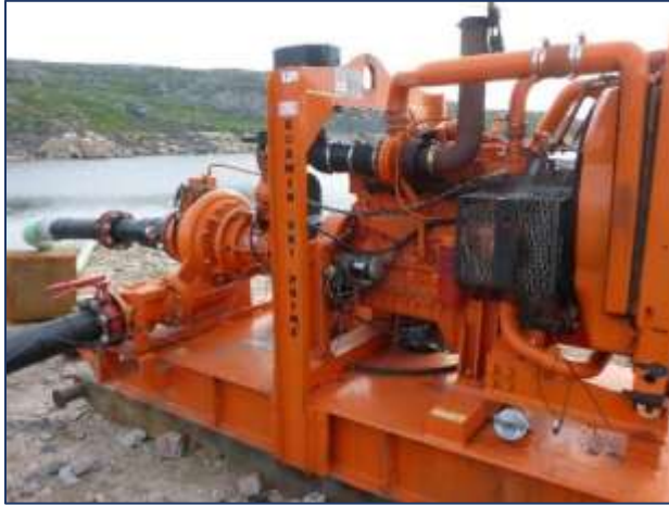
Photo 2. Typical pump used for dewatering cells (West Dam).
