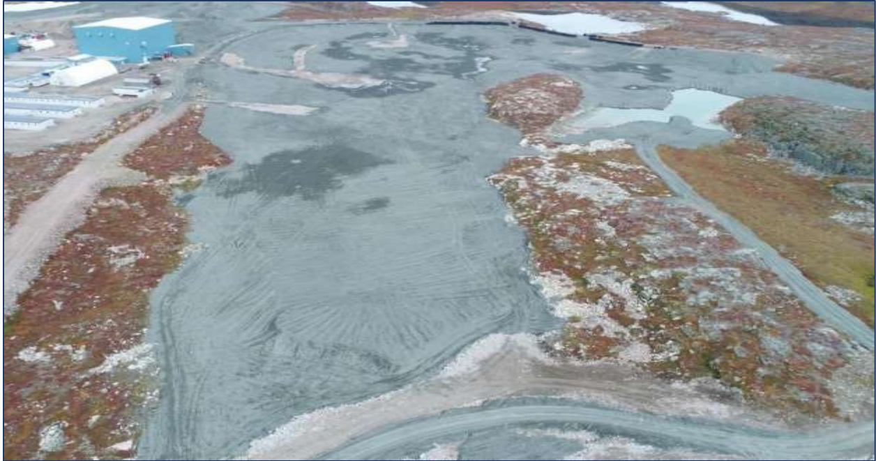
Photo 31. Overview of PKCA; rock drain channels visible; south pond (right side of photo) closed in by coarse PK; bypass road upstream of Dyke A at bottom of photo (looking east).
