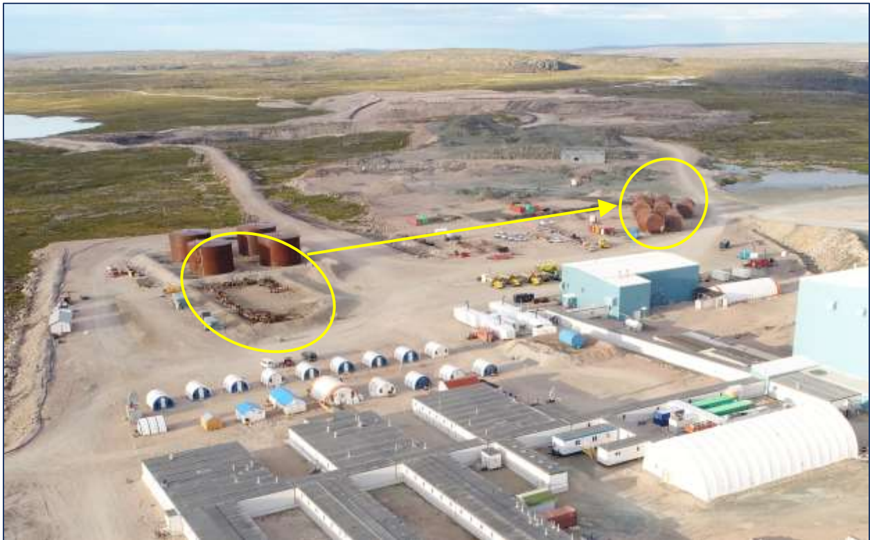
Photo 37. Fuel tanks #1 to #8 cleaned and moved from Phase 1 tank farm to laydown area (looking north).
