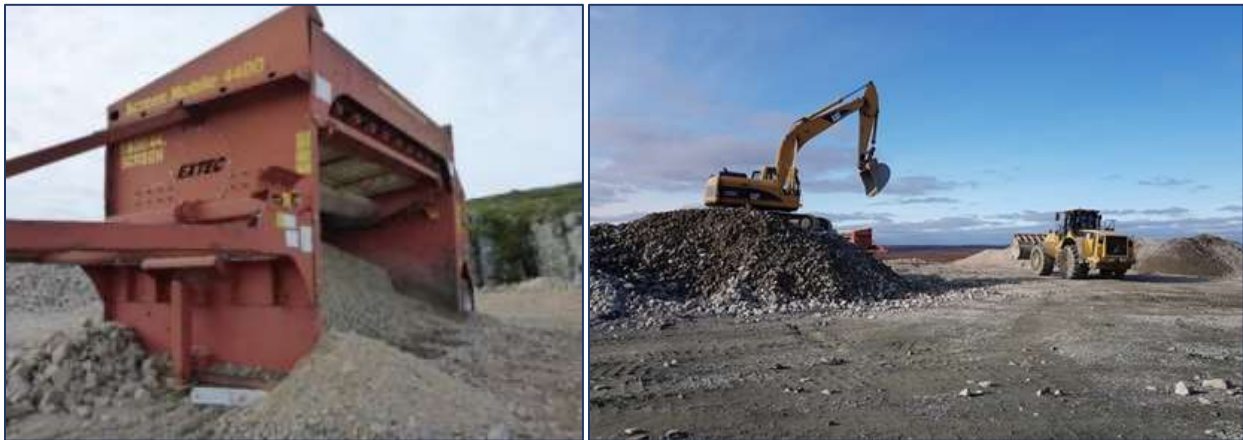
Photo 45. Screening plant making riprap near West Dam. Photo 46. Stockpiled riprap near the coarse PK stockpile.
