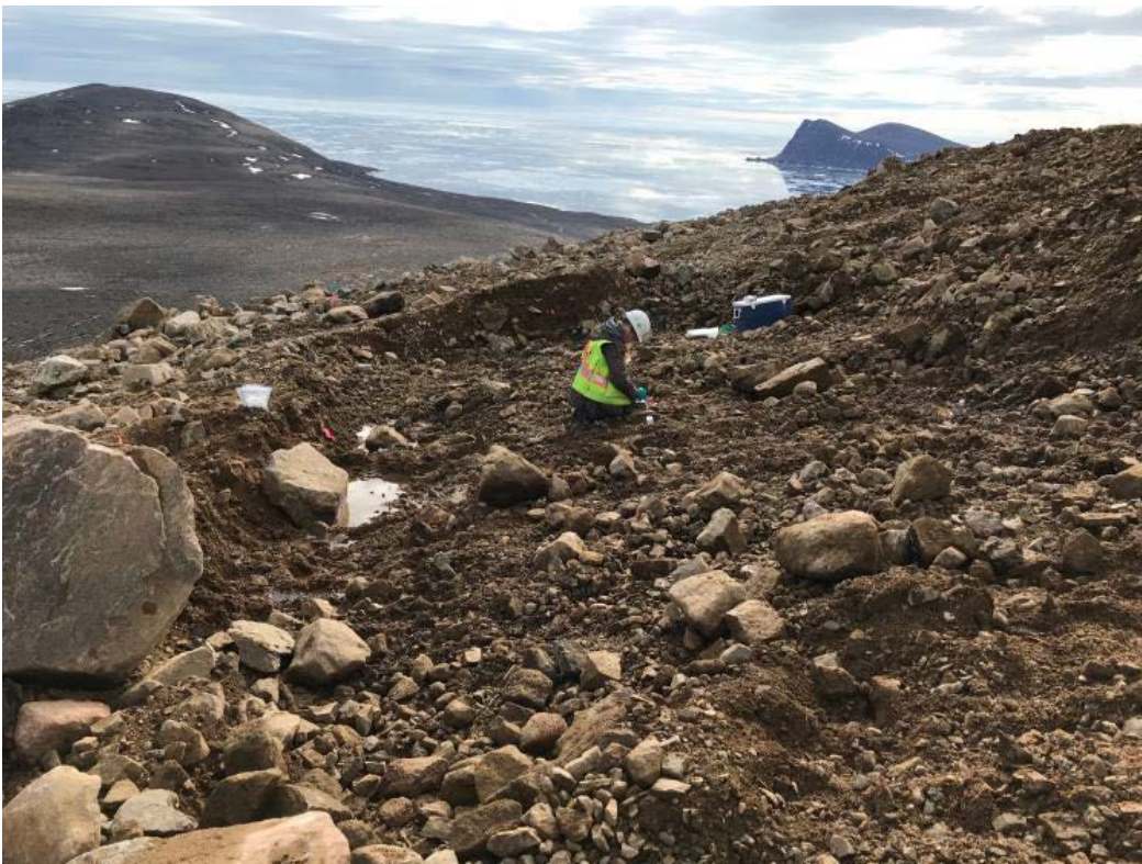
Figure 6. Environmental Inspector completing confirmatory sampling at the base of a contaminated soil excavation within APEC 9-1 at FOX-D Kivitoo.
