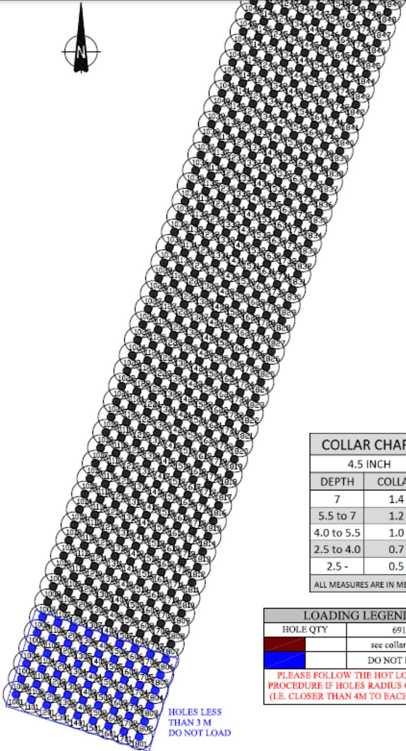
HOLES LESS THAN 3 M DO NOT LOAD
