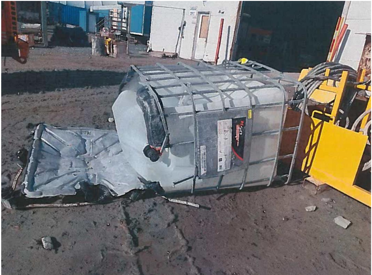
Figure 2: Damaged DEF tote outside of workshop, prior to clean-up.
