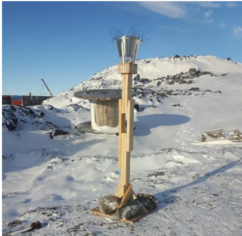
Figure 2. Dustfall sampling stand at the Meliadine site.
