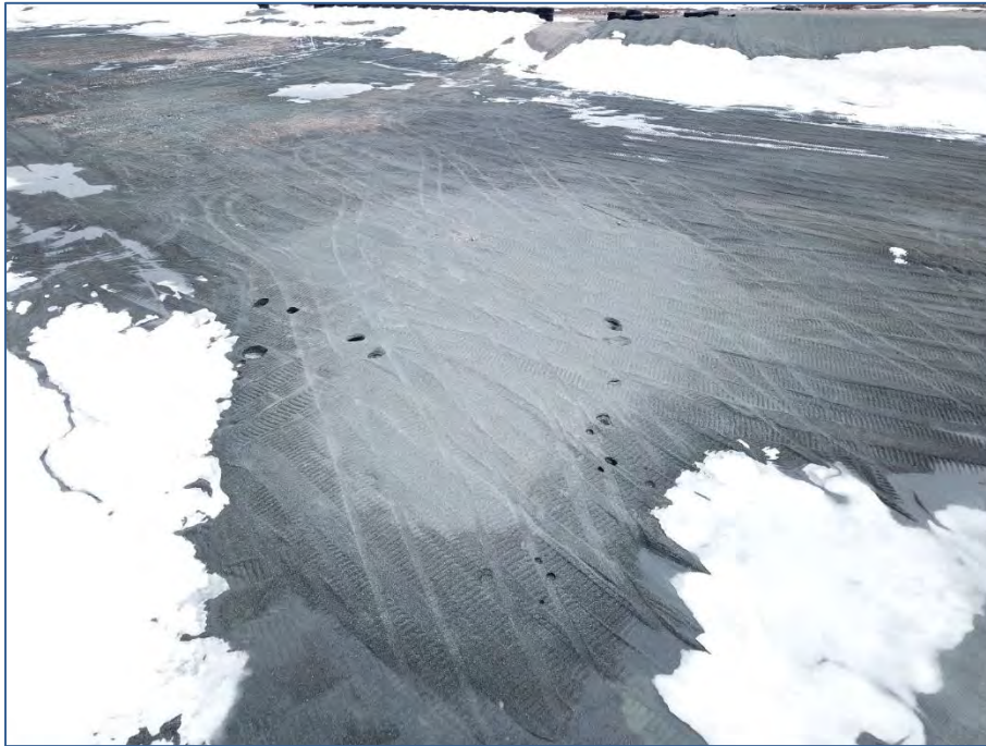
Photo 21: June 6, 2018 PKCA Cover, Southeast PKCA – 2018 aerial photo of potholes.
