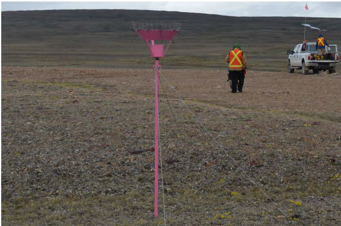
Photo 1. Dust fall collector sampling apparatus, July 10, 2013.
