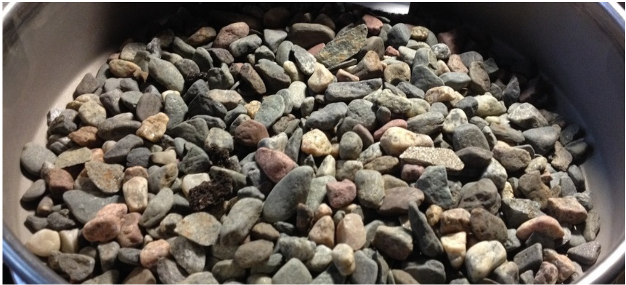
Figure 8-2: Coarse gravel fraction (retained on 10 mm sieve) from test pit S2 at KM 8.0 deposit, demonstrating sub-angular to rounded particles of hard, resistant rock that have been transported long distances and/or continually exposed to years of wave action.
