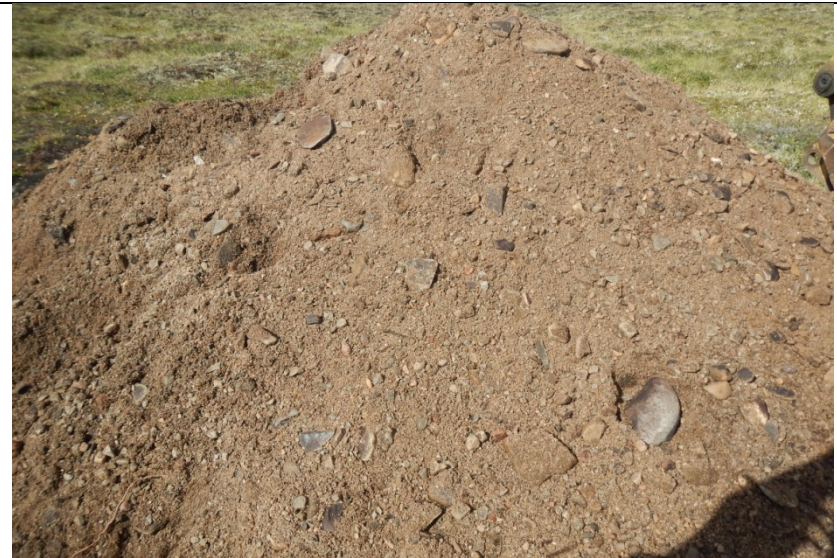
KM 19.0 on Diane River Road - Test Pit J5-S2 : Gravelly sand (similar to TP J5-S1), trace cobble and trace shale fragments in gravel component. Permafrost at 3'10". No silty till encountered.
