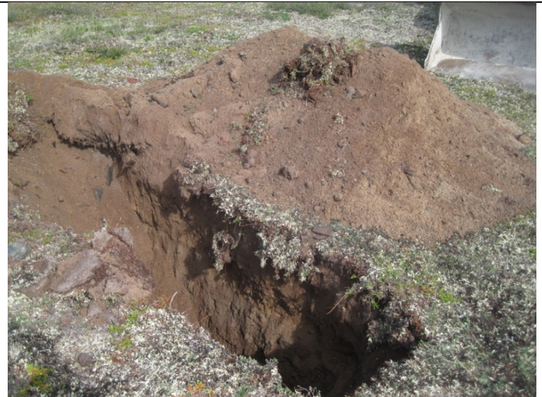
KM 19.0 on Diane River Road - Test Pit J5-S10 : Reddish-brown sand with little gravel. Permafrost at 3'10".
