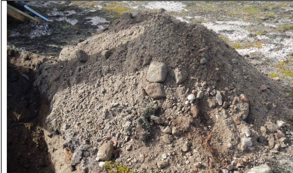
KM 19.0 on Diane River Road - Test Pit J5-S3 : Gravelly sand with cobble. Very similar to J5-S1 and S2. Permafrost at 3'11". No silty till encountered.
