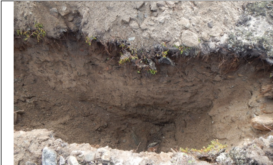
KM 19.0 on Diane River Road - Test Pit J5-S1 : Gravelly sand (medium grain). No flat shale fragments noted. Water table encountered at 5'0" below grade atop permafrost. No silty till encountered
