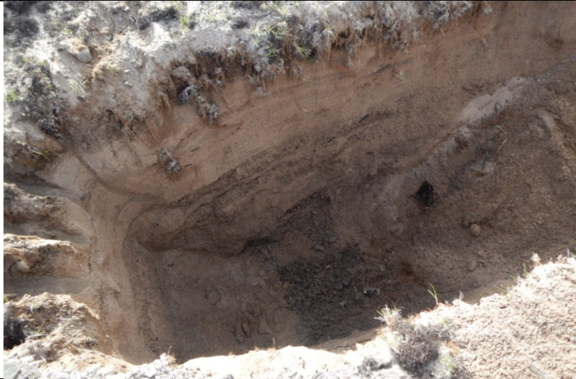
KM 19.0 on Diane River Road - Test Pit J5-S5: Stratified sand with trace to some gravel. Very similar to material in J5-S4 but even higher sand component (~70%). Permafrost at 4'10". Increased gravel can be seen at the permafrost table.
