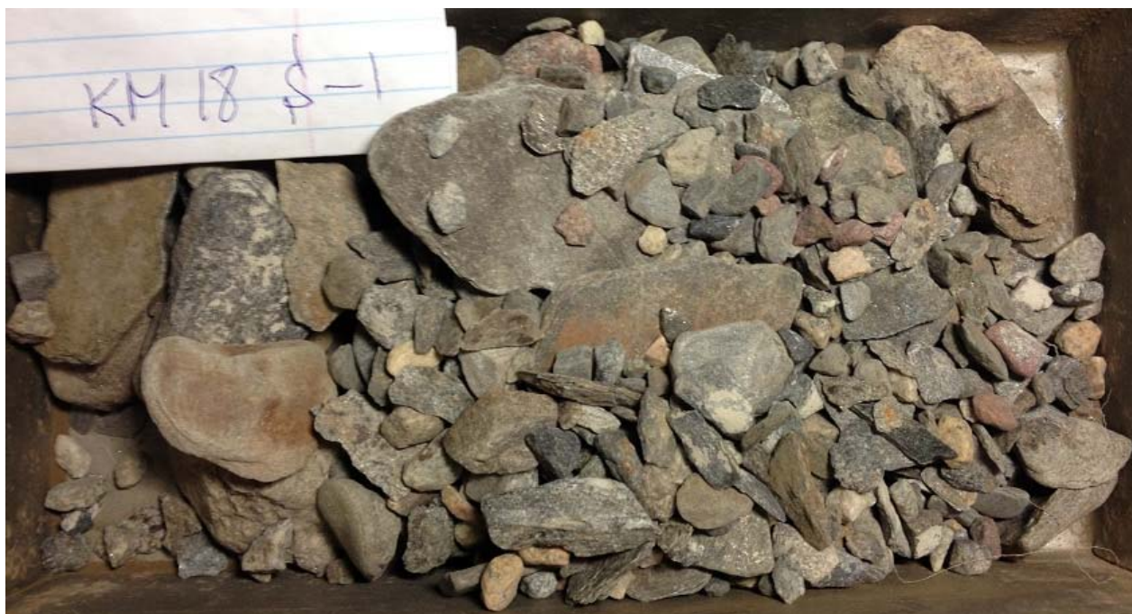
Figure 8-3: Coarse gravel fraction (retained on 10 mm sieve) from test pit S1 at KM 18.0 deposit, demonstrating angular to sub-angular particles of hard, resistant rock mixed with roughly 20% flat, elongated shale and/or slate.
