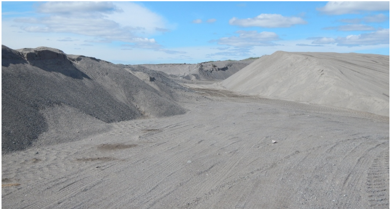
Figure 6-9: Screened stockpiles of fine gravel (left) and clean sand (right) in the Meliadine Pit (Photo: July, 2016).
