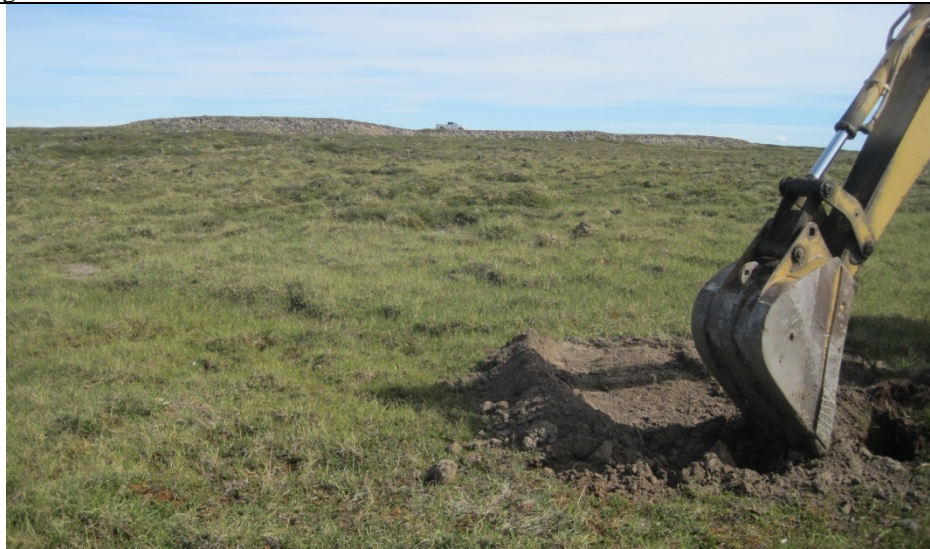
KM 19.0 on Diane River Road - Test Pit J5-S11 : Grey silt with trace to some sand. Stopped test pit at 2'4". Note distant gravel ridge below truck (area of J5-S7)
