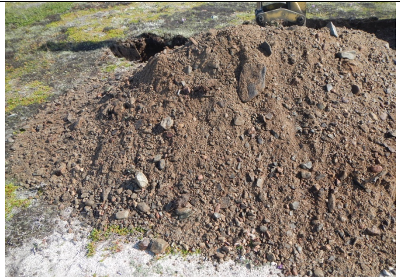
KM 19.0 on Diane River Road - Test Pit J5-S12 : Sandy gravel with trace cobble. Generally minus 4" gravel. Appears well graded. Minimal shale component (<10%). Permafrost at 4'6". No silty till encountered.
