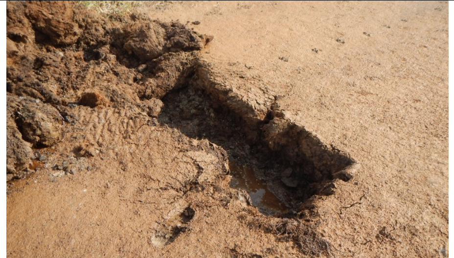
KM 19.0 on Diane River Road - Test Pit J5-S8: This test pit in the bottom of a dry pond revealed sandy gravel similar to that of J5-S6 beneath 21" of peat and silt. Permafrost was shallow at 24" with groundwater perched atop it in the gravel.
