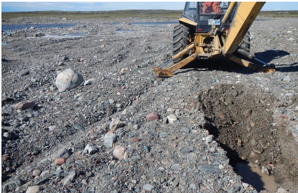
Figure 6-6: Excellent course aggregate (~40,000 m 3 ) remaining alongside and beneath the small middle lake at the north end of the existing Diane Pit (Photo: July, 2016).
