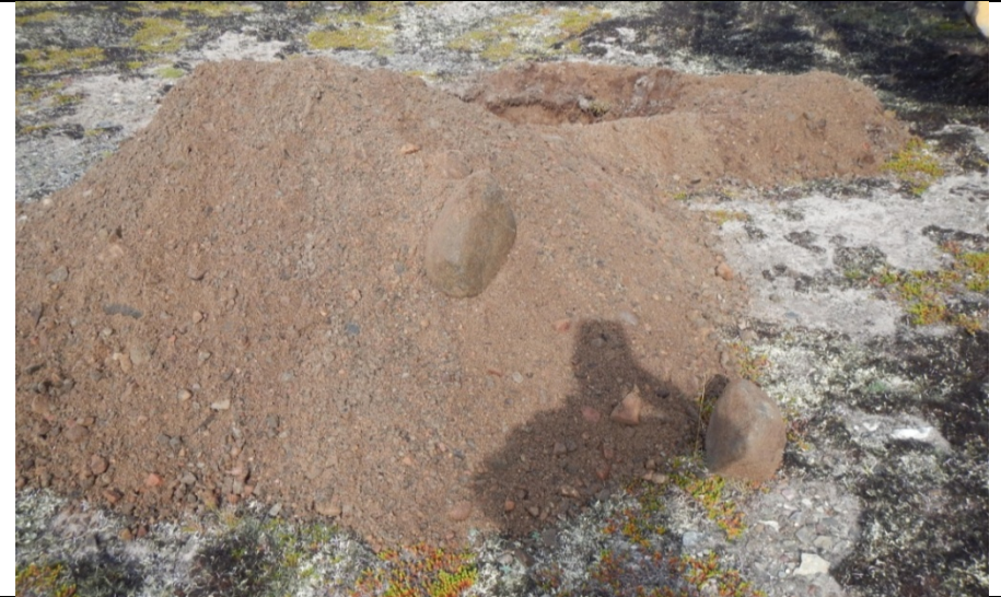
KM 19.0 on Diane River Road - Test Pit J5-S6: Sandy gravel with trace cobbles. Appears well graded. Generally minus 2" gravel. Permafrost at 4'0". No silty till encountered.
