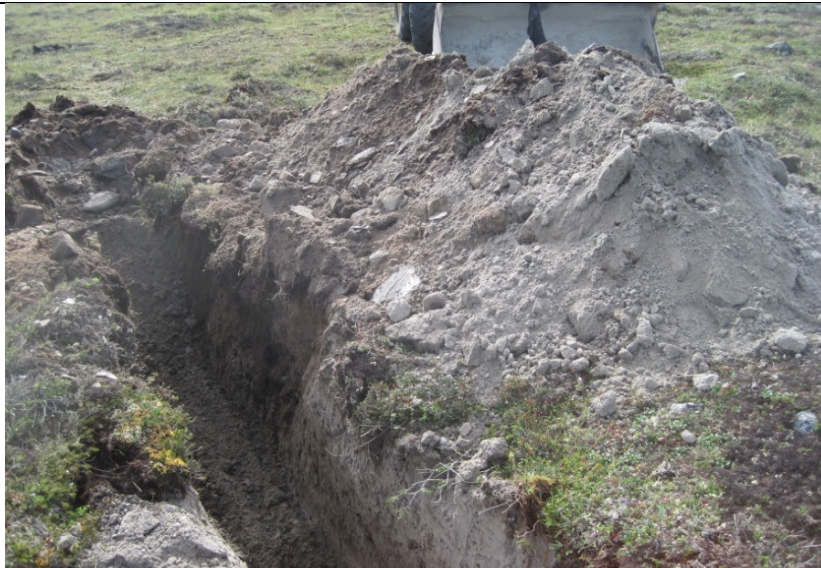
KM 19.0 on Diane River Road - Test Pit J5-S9 : Grey sandy silt with trace-little gravel and cobble. Permafrost at 3'10".
