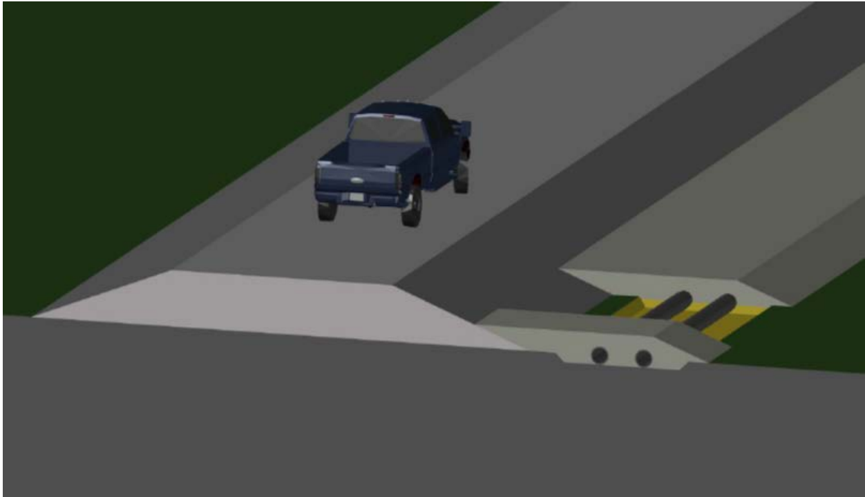
Figure KivIA-IR-8a. Conceptual design of waterline cover on the east side of the All Weather Access Road.
