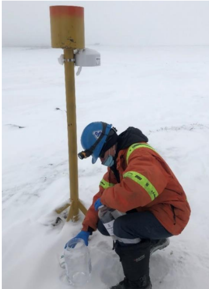
Photo 69: Dust and NO 2 sampler at station DF-6
