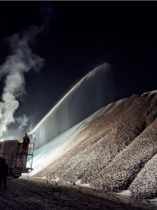
Photo 1. Application of DusTreat® onto ore stockpiles at Milne Port during pilot application in November 2020.
