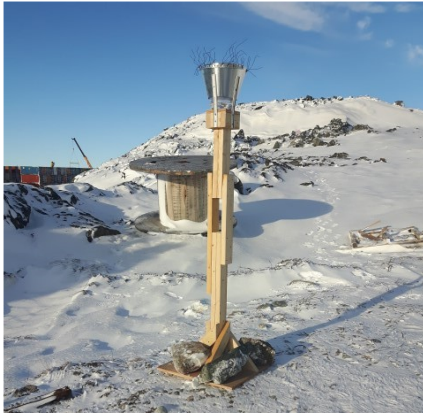
Figure 2. Dustfall sampling stand at the Meliadine site.
