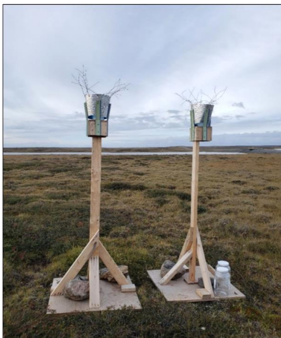
Photo 4-1-1: Example of a dustfall sampling station.
