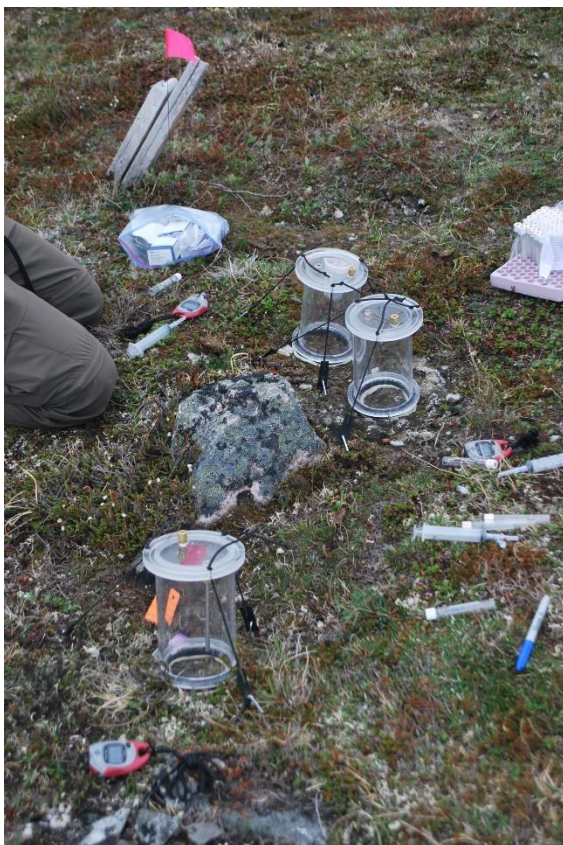
Figure 18. Static vented gas flux chambers on BSCs at drilling wastes from 1997/1998. Gas flux was sampled every 15 minutes over a 1 hour period to determine in-situ \text{CO}_2 , \text{N}_2\text{O} and \text{CH}_4 .
