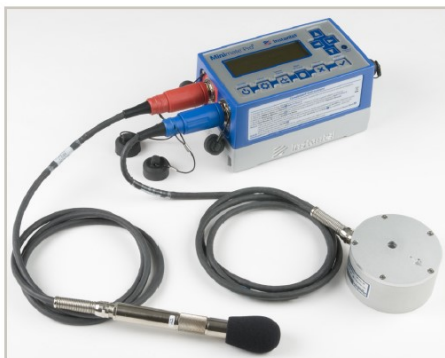
Figure 1. Minimate Pro4 components
