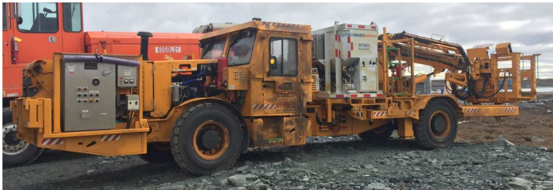
Figure 3-3 Underground Emulsion Charger – Dyno Loader
