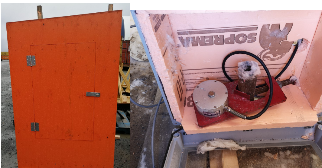
Figure 6. Surface Installation (Shelter & installation inside)
