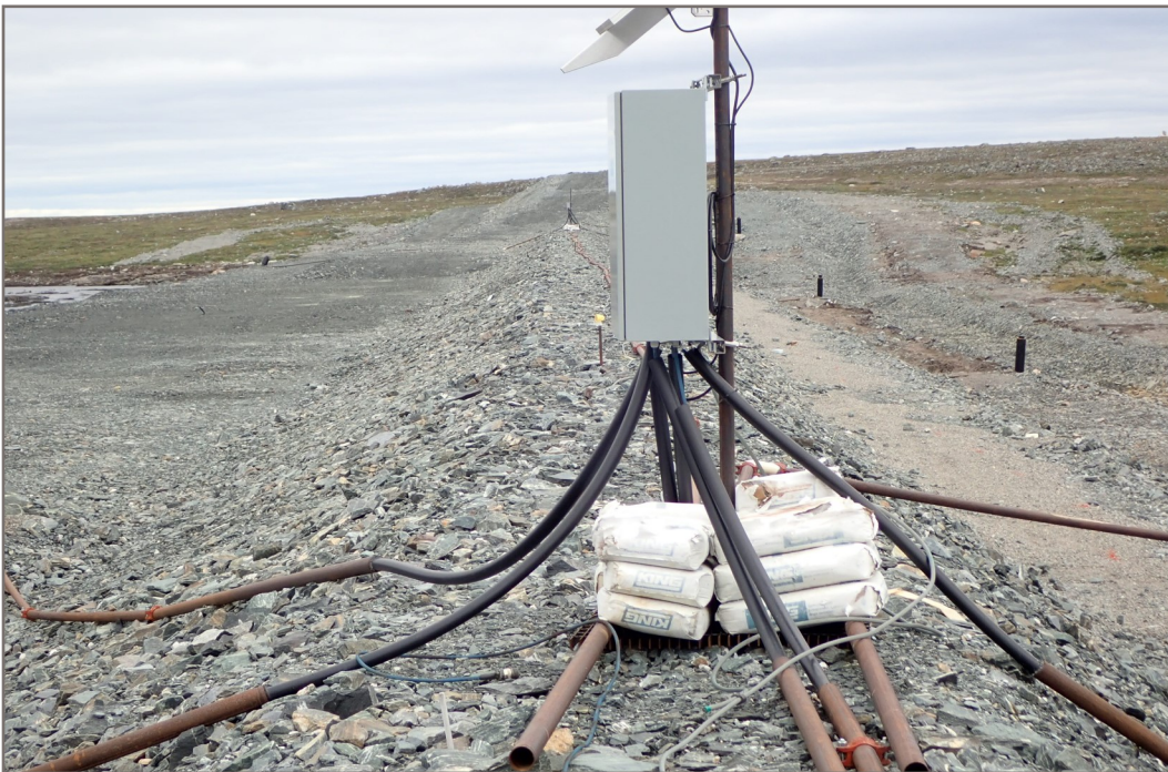
Photo 10: Dike D-CP1 - Dike crest, data acquisition terminal for GTCs
