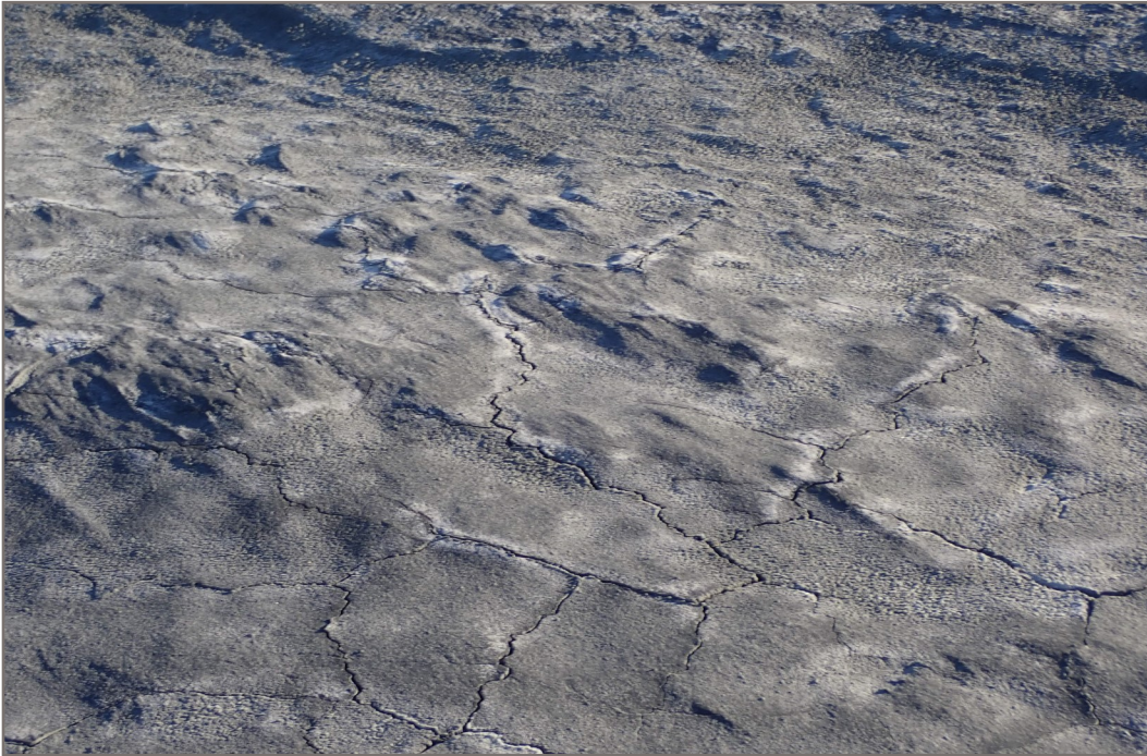
Photo 9: TSF - Desiccation of tailings, reported to be placed approximately three months prior.
