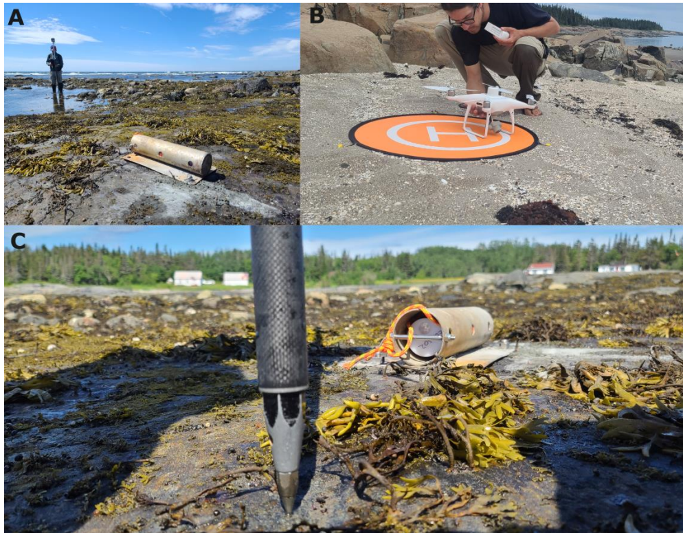
Figure 3. Installation of pressure sensors for wave and water level measurements (A), drone surveys (B) and high-resolution vertical measurements of the beach topography using RTK-GPS (C). These works will be conducted in summer 2021 to validate the preliminary assessment.
