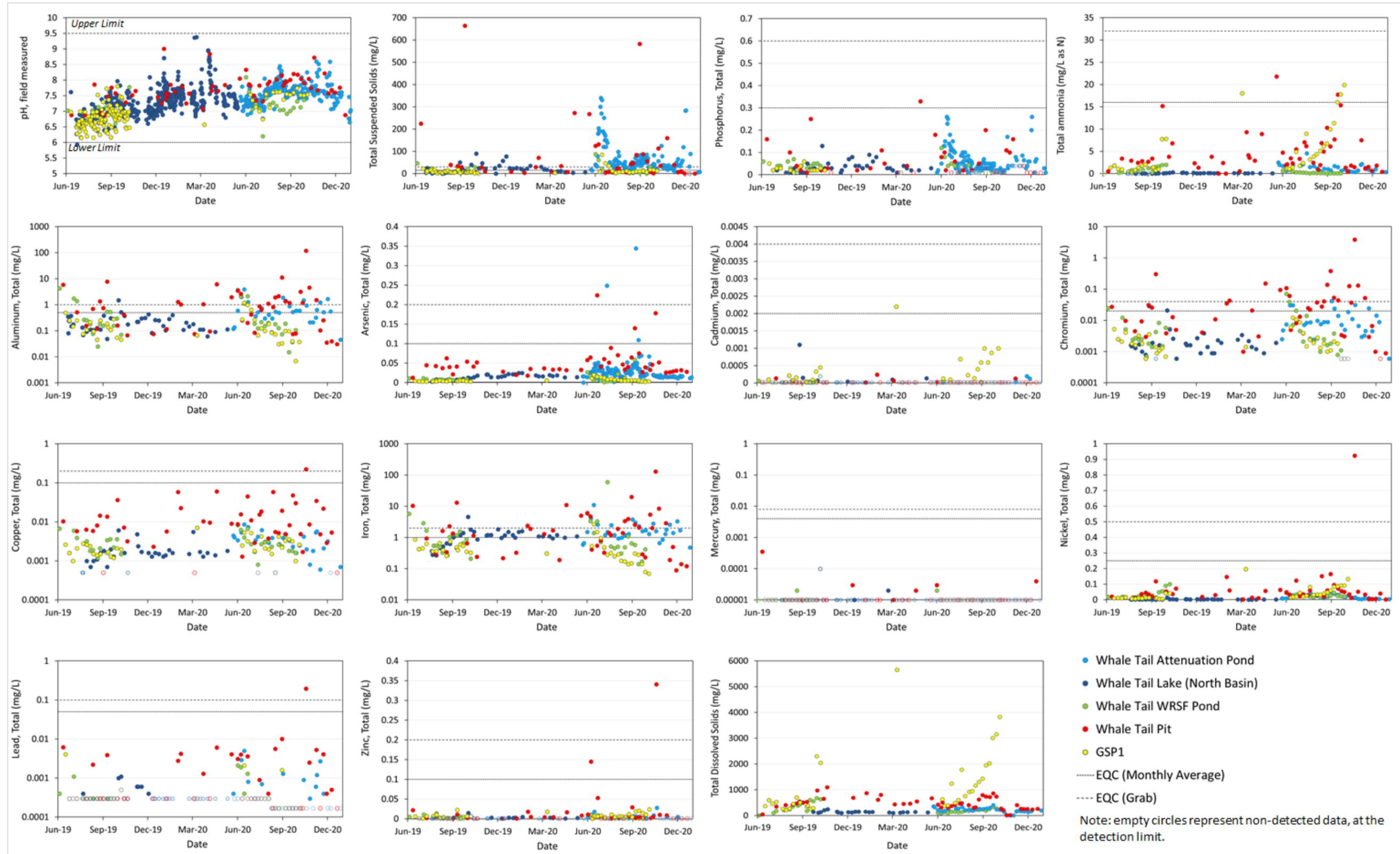
Figure 6: Monitored concentrations of constituents compared to their respective Effluent Quality Criteria
