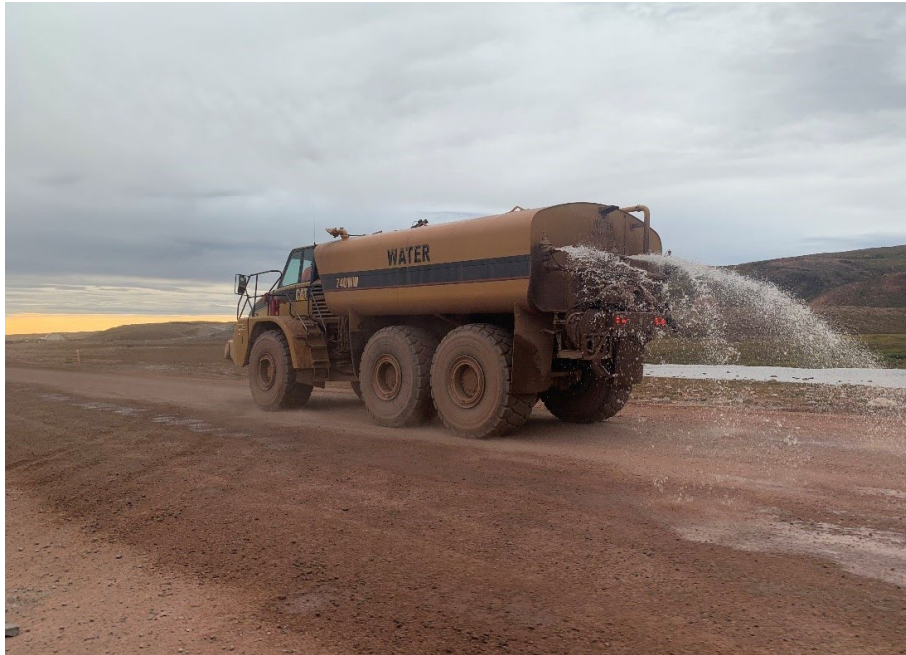
Photo 10 : Dust Suppression Water Truck on Tote Road - August 2020
