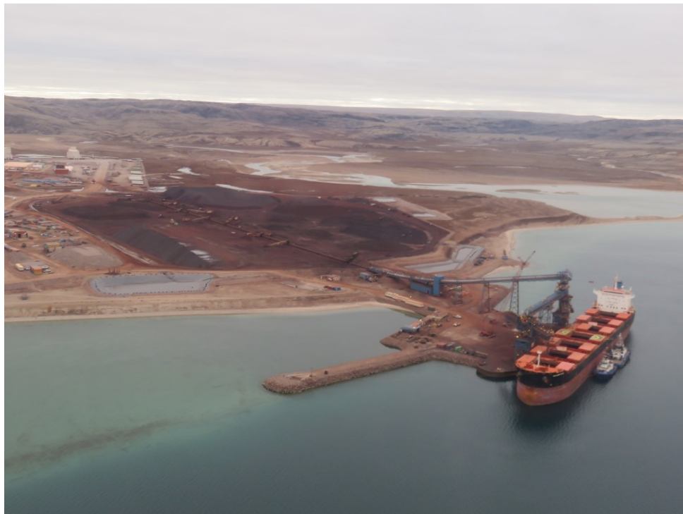
Photo 5: Vessel Being Loaded with Iron Ore at Milne Port using Ship Loading Conveyors
